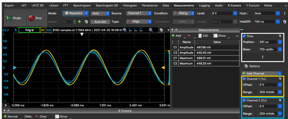
Figure 63: Output Buffer Transient Response ( V_{in} = 500\text{mV} , 440Hz)
