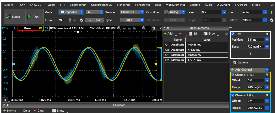
Figure 61: Input Buffer Transient Response ( V_{in} = 500\text{mV} , 440Hz)
