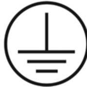
Figure 29: Earth Ground Symbol
